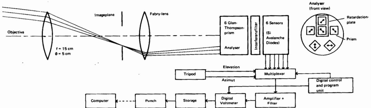
● Fig. 2. Schematic representation of the polarimeter
