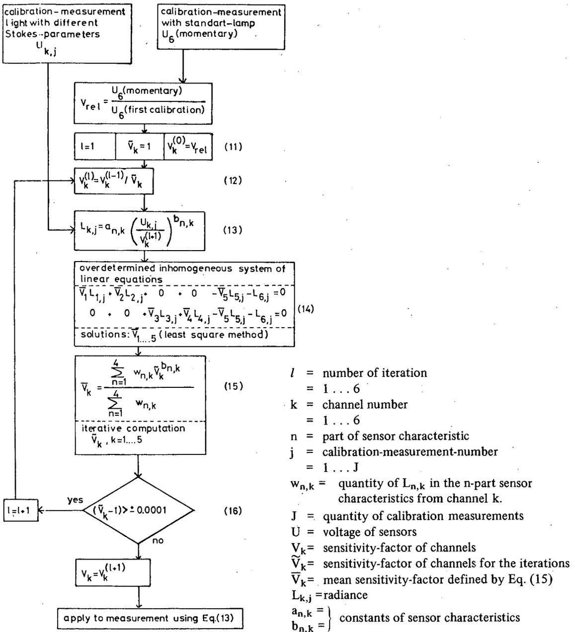
• Fig. 4. Scheme of channel sensitivity computation
