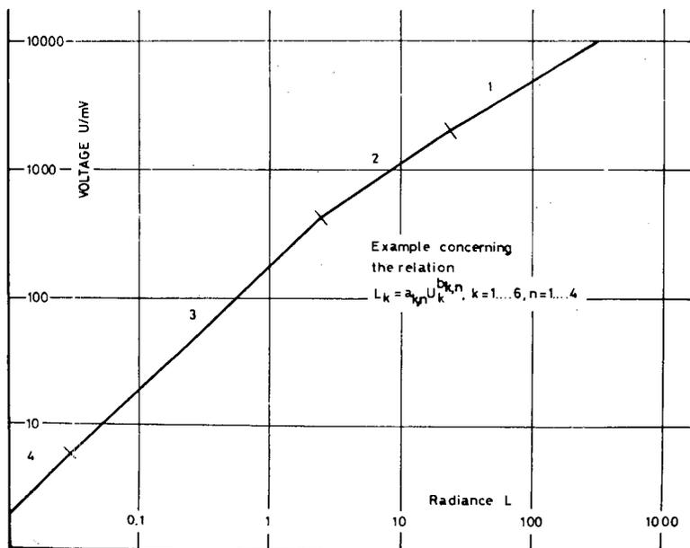
● Fig. 3. Typical characteristics of one of the Si-avalanche diodes
